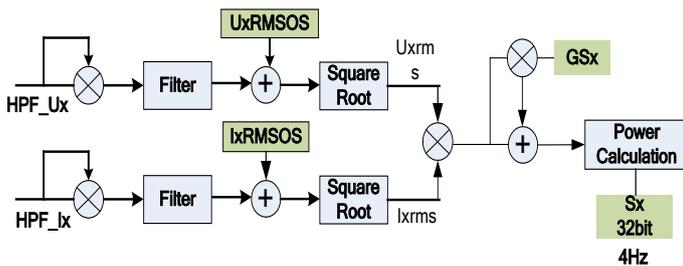
Figure 2-3 Split Phase Apparent Power
