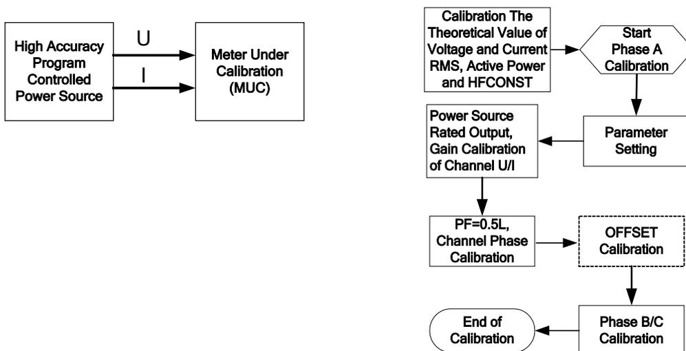
Figure4-1 Calibration Flow
