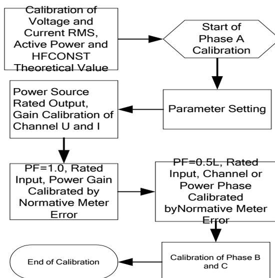
Figure 4-3 Pulse Method Calibration Flow
