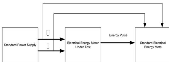
If provided with the program controlled power source with general accuracy, but with the high level of the normative meter, they may take the pulse calibration method as shown in the figure left into account.
