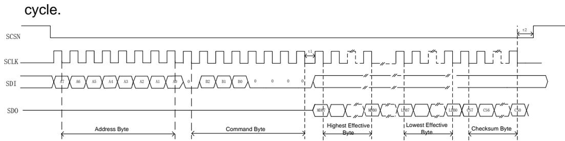
Figure 5-2 SPI Reads Timing
