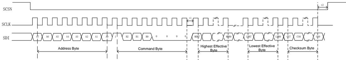
Figure 5-1 SPI Writes Timing
