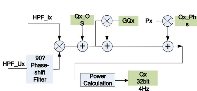
Figure 2-2 Per-Phase Reactive Power
