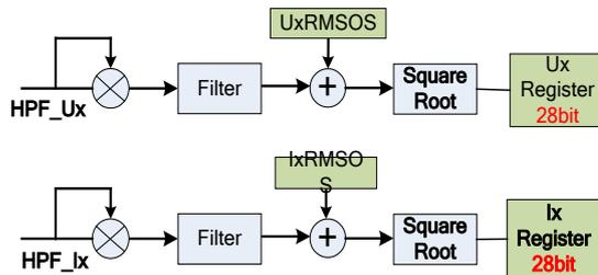
Figure 2-4 Voltage and Current RMS
